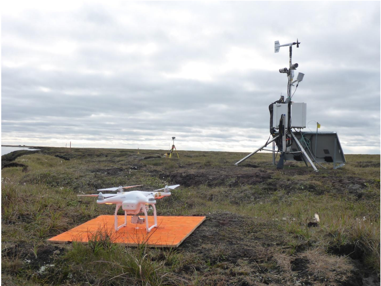
Figure 29. DJI Phantom 3 unmanned aerial vehicle ready to conduct the aerial survey of FIB.
