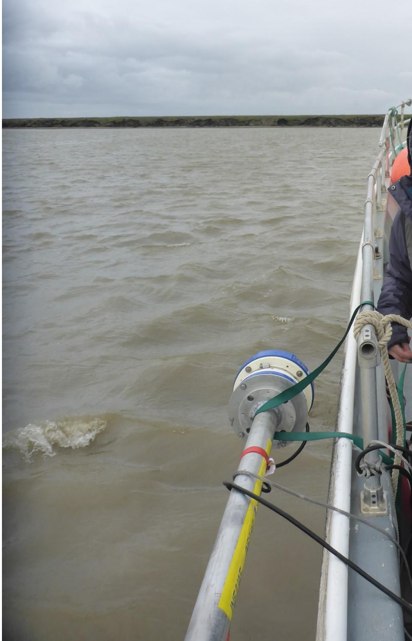
Figure 11. 600 kHz RD Instrument Sentinel Workhorse ADCP pole mounted off the R/V Ukpik
