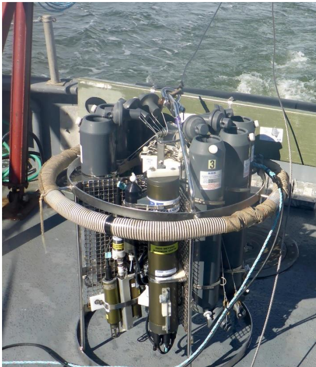
Figure 23. Seabird Electronics SBE25+ equipped with an SBE 55 water sampler and ancillary sensors.
