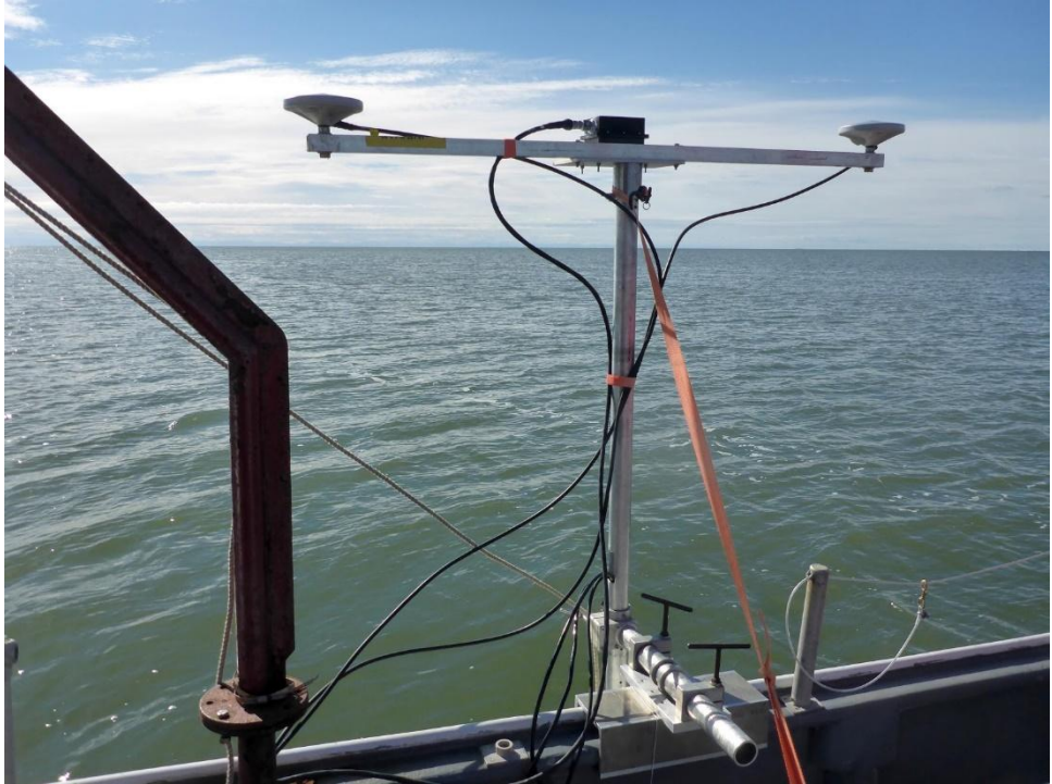
Figure 10. Reson 7125 Seabat Echosounder deployed with inertial motion unit (IMU) and primary and secondary antenna mounted to echosounder support beam.
