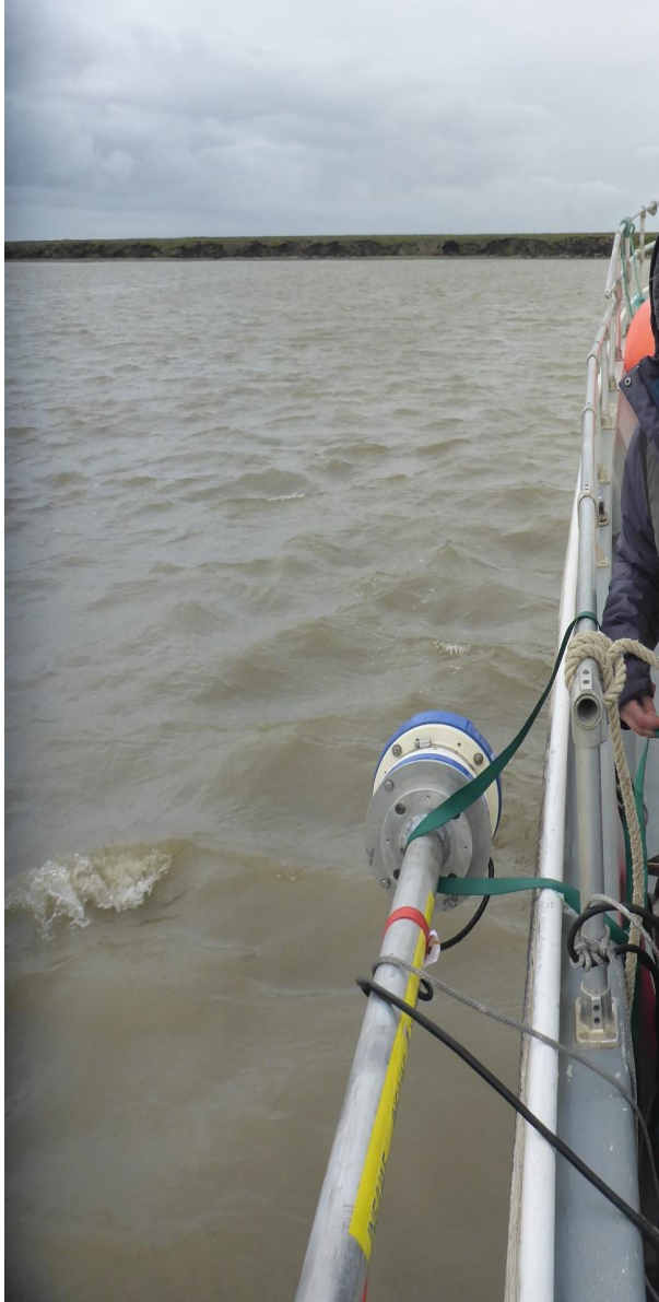
Figure 9. 600 kHz RD Instrument Sentinel Workhorse ADCP pole mounted off the R/V Ukpik
