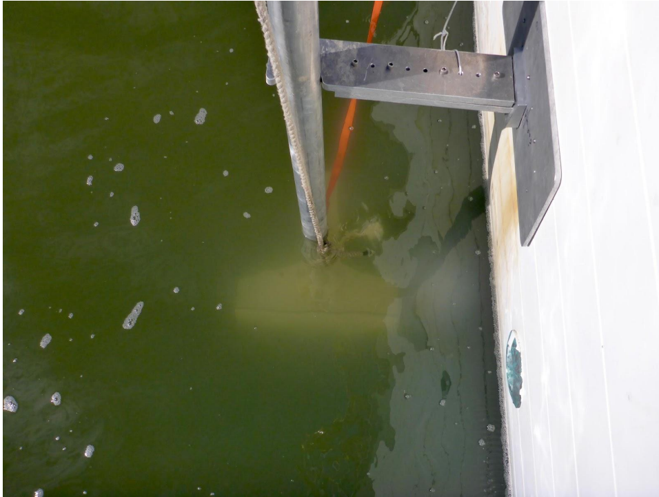
Figure 24. Reson 7125 Seabat multibeam sonar head mounted to the starboard side of the R/V Ukpik.
