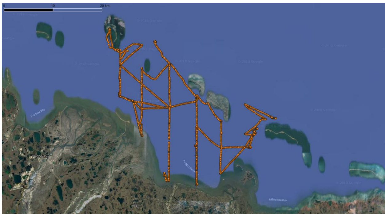
Figure 10. Coverage map of the 224 km surveyed by the Reson 7125 Seabat Multibeam Echosounder deployments
