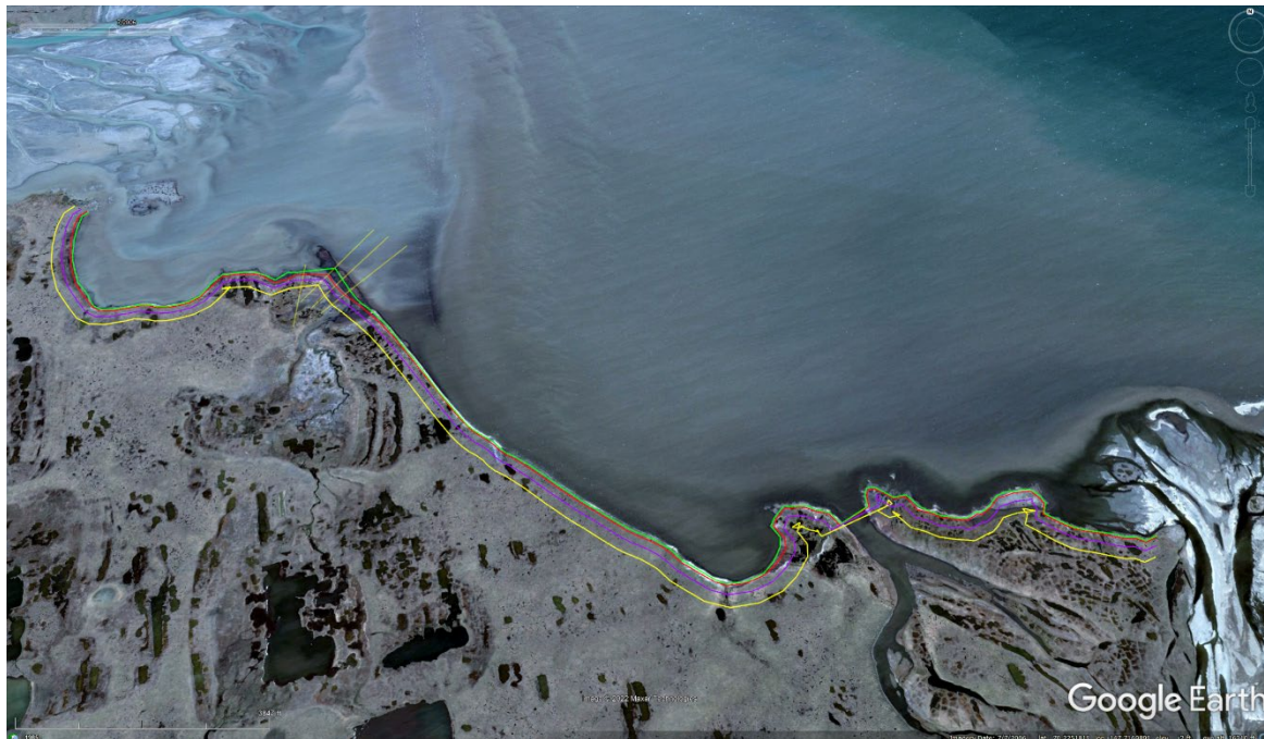
Figure 4.7 Plots of the observed 2007 (green) and 2018 (red) shorelines, along with the projected 2030 (pink) and 2049 (yellow) shoreline, for the Model 1 domain.
