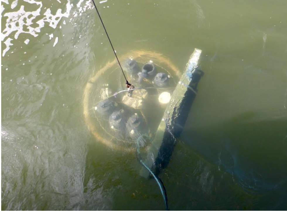
Figure 24. Seabird SBE25+ with LISST attached to carousel being retrieved at a sampling station.
