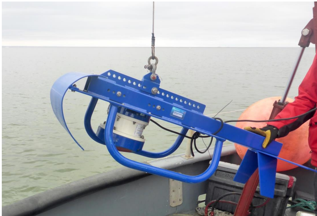
Figure 15. 600 kHz RD Instrument Sentinel Workhorse ADCP mounted on Biosonics Inc., acoustic sled.
