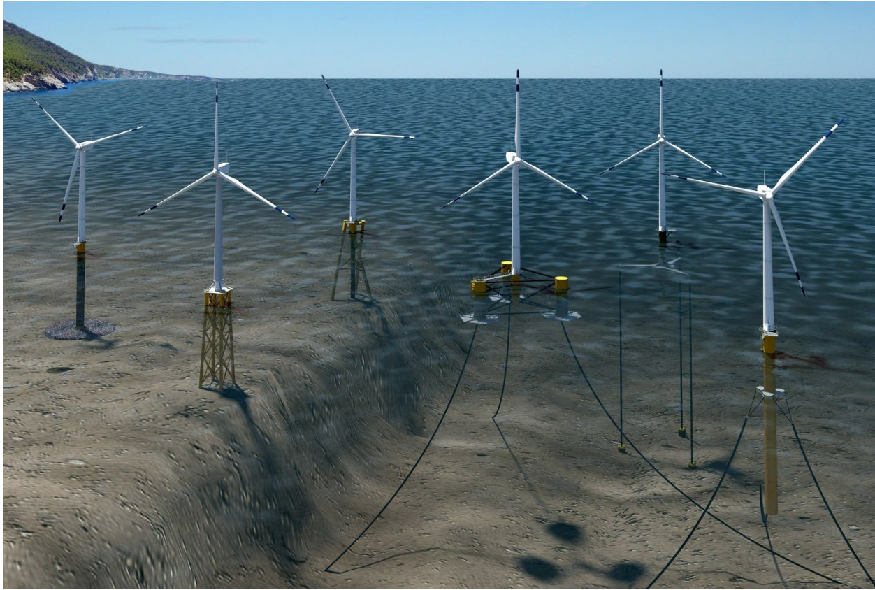
Figure 32. Offshore wind turbine substructure types
