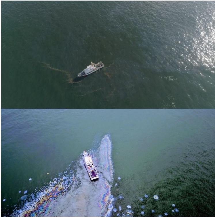
Figure 4-5. Photographs of an oil spill with and without confounding glare Top depicts oil with glare. Bottom is at a different angle with a multispectral camera. From O. Garcia, WaterMapping.
