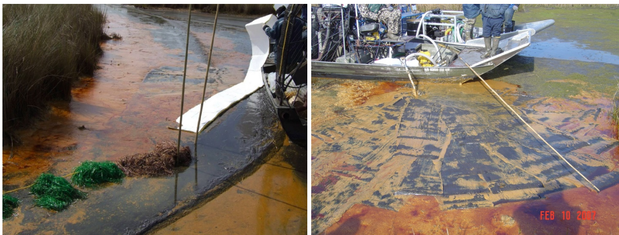
Figure 8-6. Emulsified condensate on muddy tidal flats after the 8,500 bbl 2007 Bayou Perot spill in Louisiana
