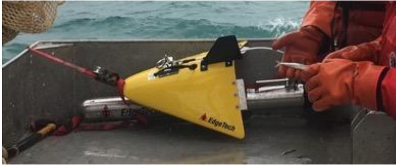
Figure 27. Edgetech 4125 side scan sonar equipped with depressor wing.
