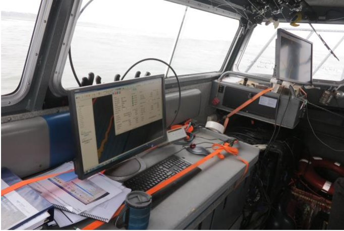
Figure 36. Setup of the Reson Seabat operating system in the cabin of the F/V Quest.
