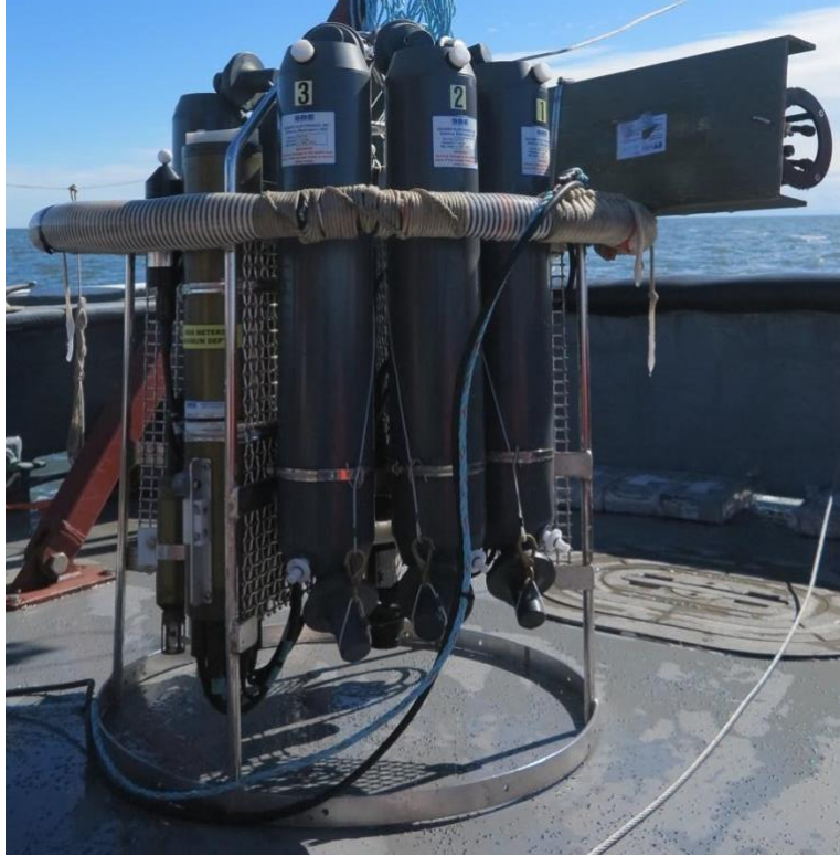
Figure 32. The Seabird 25 CTD and SBE55 water sampler with the LISST100X attached to the frame.
