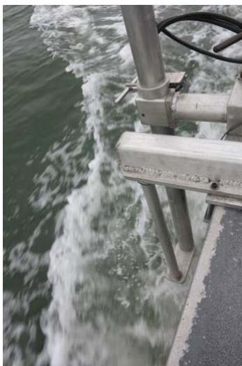
Figure 35. Vertical pole stabilizer for the multibeam pole mount on the starboard gunwale of the F/V Quest.
