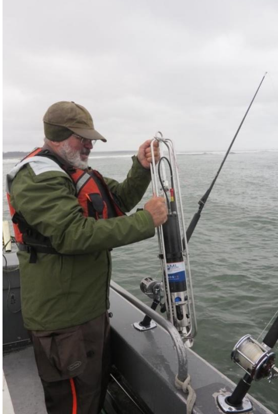
Figure 39. The AML CTD+Tu being deployed from the F/V Quest.
