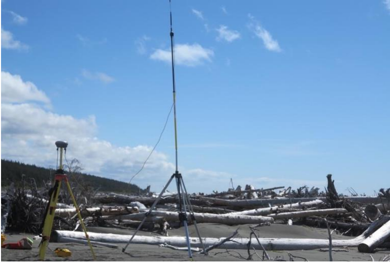
Figure 40. The Trimble GNSS base station set up to broadcast real time kinematic position corrections to the GNSS rover used to survey beach elevations.
