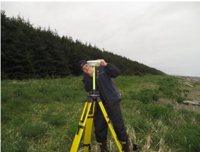
Figure 37. Setting up the Trimble R8 base station broadcasting real time kinematic corrections to the F/V Quest for the multibeam survey.
