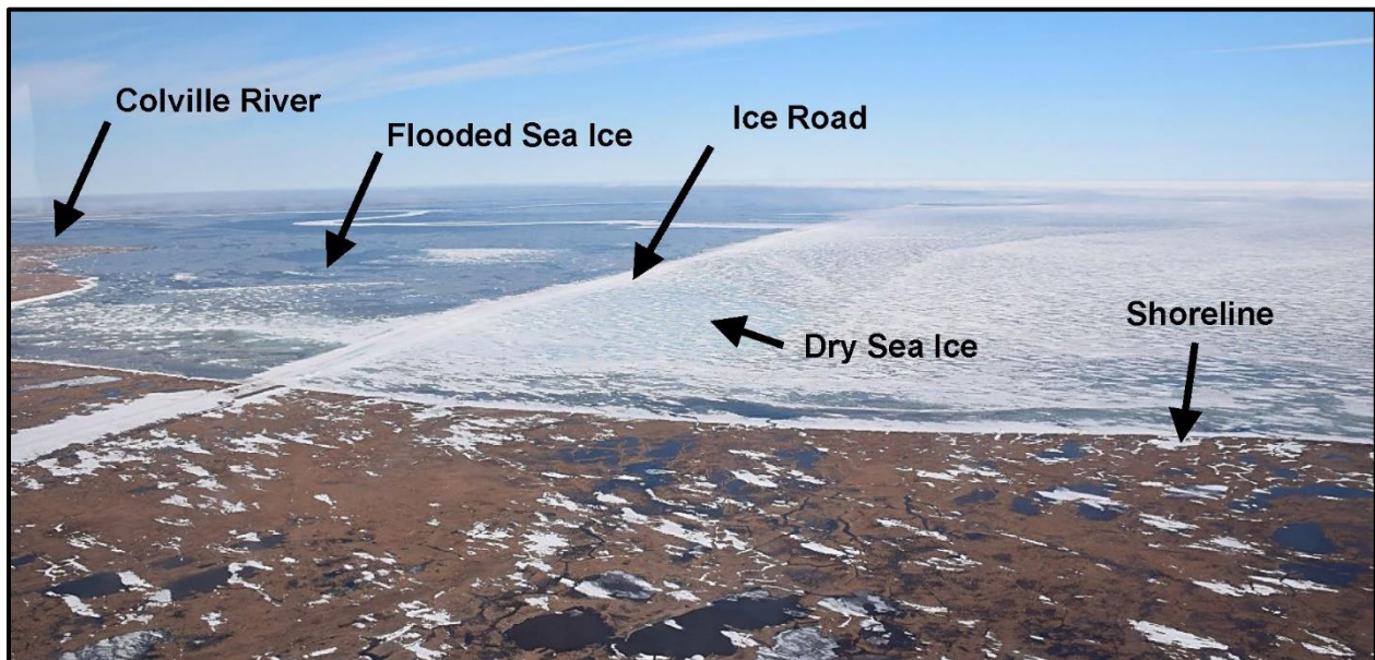
Figure 8. Overflow from the Colville River impeded by an ice road
