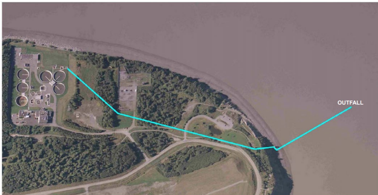
Figure 23. Route of outfall pipe into Cook Inlet for the Anchorage John M. Asplund Wastewater Treatment Facility.
