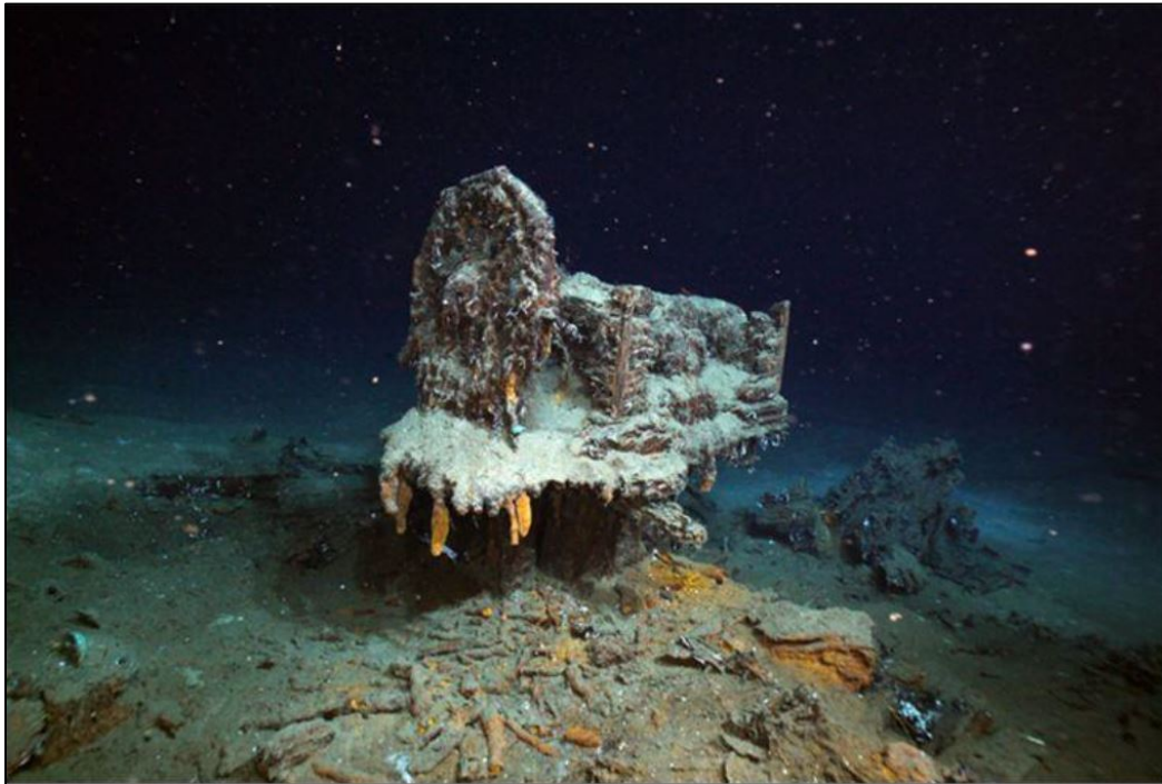
Figure 15. The 7,000 Foot Wreck's helm, showing the wheel, exposed wheel-box, and rudder case From Brooks et al. 2016.
