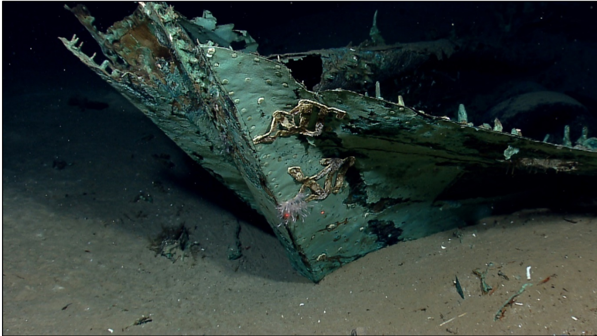
Figure 13. Bow of Monterrey A, showing lead Roman numeral draft marks over copper hull sheathing Image courtesy of the National Oceanic and Atmospheric Administration.
