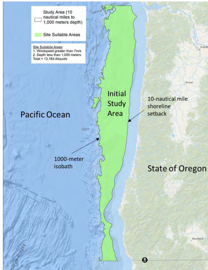
Figure 3. Initial study area defined by the study site selection team. “Site Suitable Areas” denote technical viability for the purposes of this study. Image adapted from Parametrix
