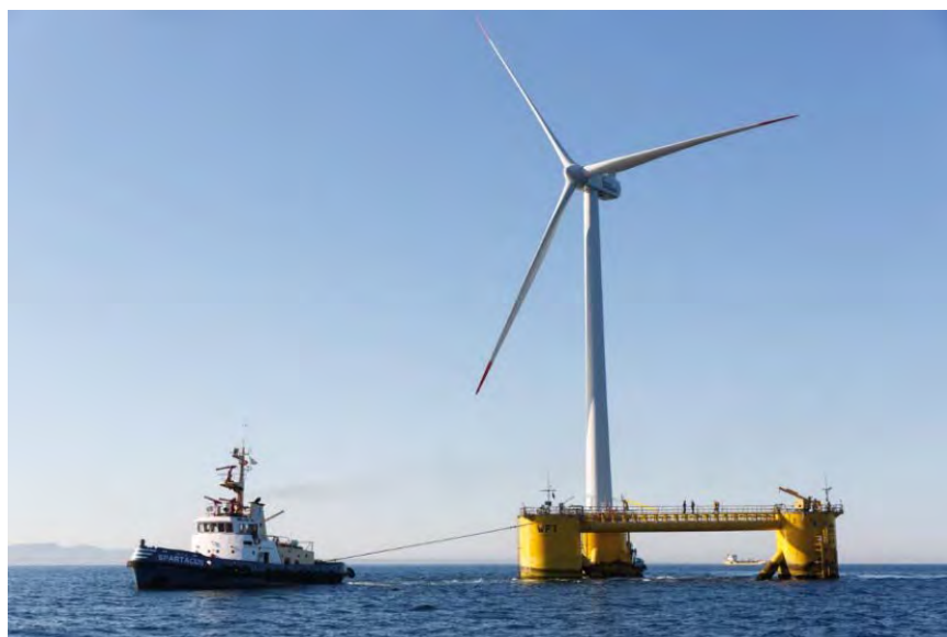
Figure A-1. Principle Power, Inc. semisubmersible with mounted turbine. Photo courtesy of Principle Power, Inc.
