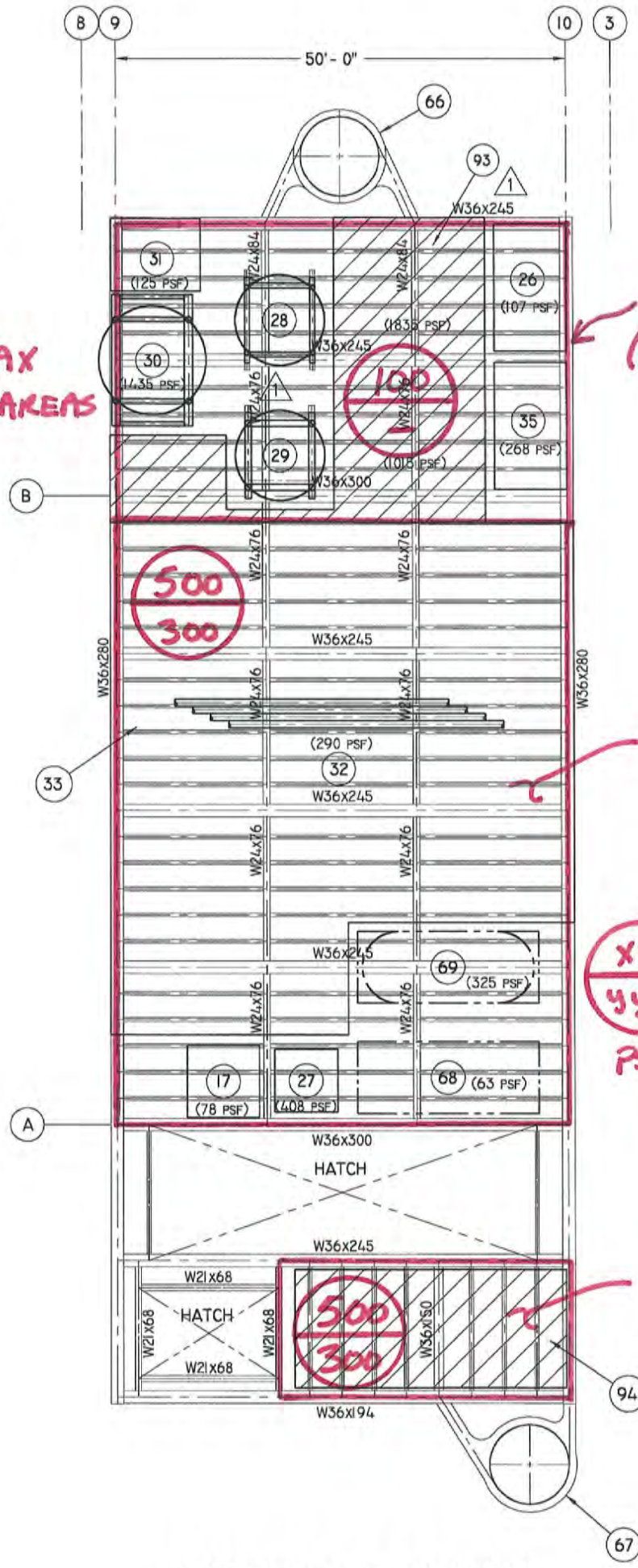
PLATFORM GAIL ROOF FRAMING PLAN T.O.S. = 104'-6" SCALE: 3/32" = 1'-0"
