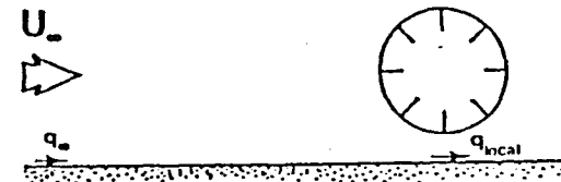
Fig. 2.33 Definition sketch of q_{\infty} and q_{\text{local}} .
