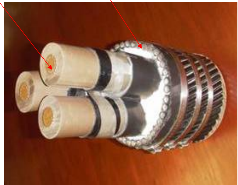
35 kV Kerite Cable Installed in 1993
