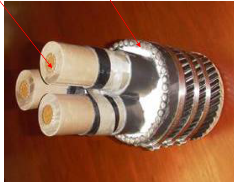
35 kV Kerite Cable Installed in 1993
