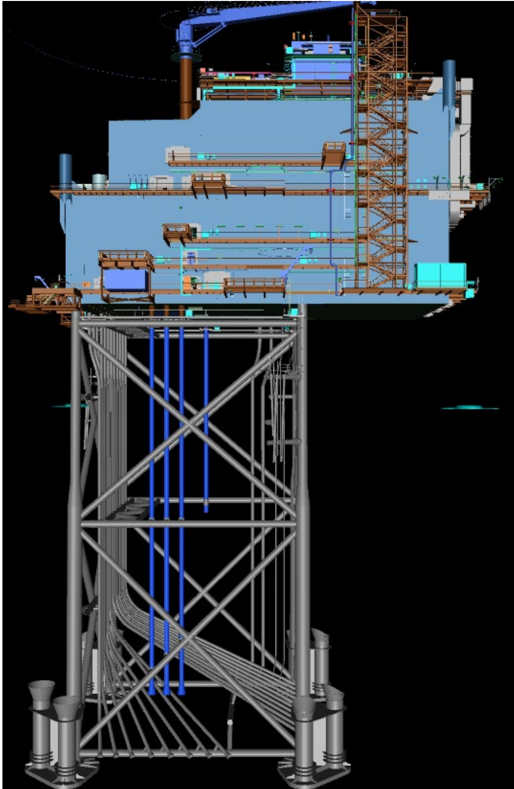
Figure 18. Indicative representation of the cooling water intake (3 longer blue caissons) and discharge (single shorter blue caisson)
