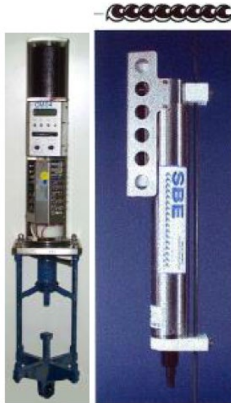
Figure 2-4. CM-04 Acoustic Current Meter (Left) and Seabird SBE37 CT Logger (Right)
