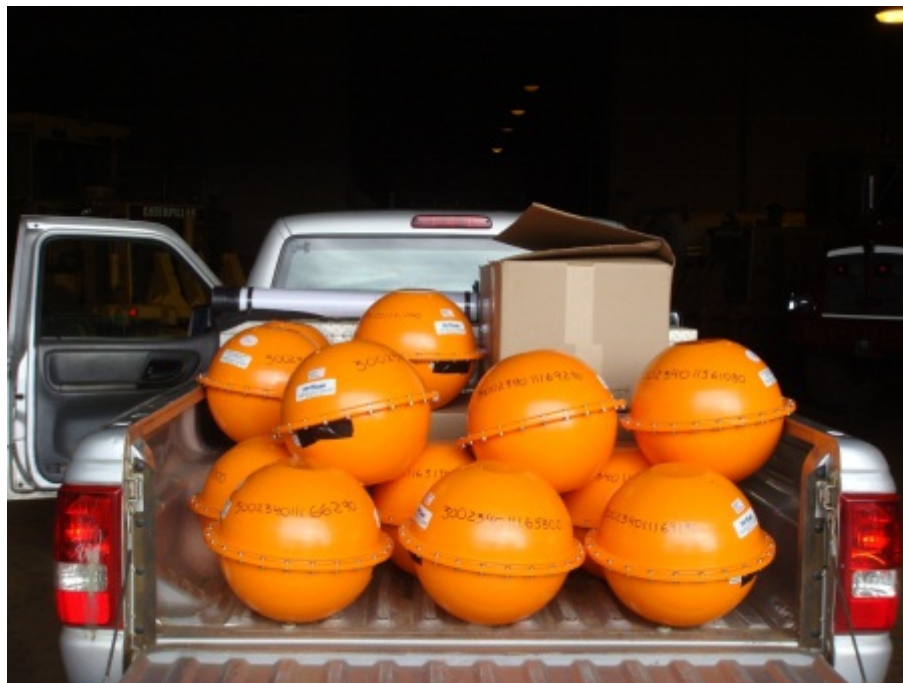
Figure 5. iSphere surface drifters (manufactured by Metocean).
