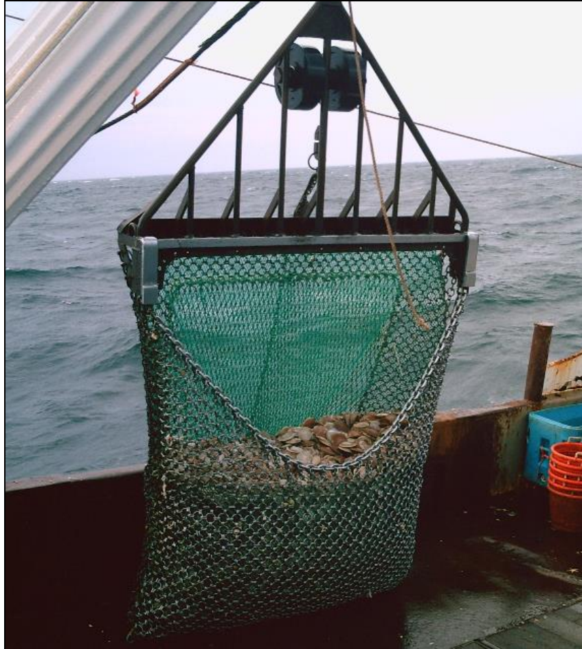
Figure 8.8-18 Commercial Scallop Dredge (Coonamessett Farm Foundation 2008)
