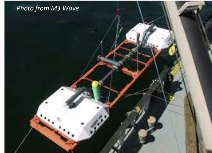
M3 – Submerged communicating volumes absorber
