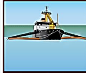
Single vessel with outrigger and containment boom
