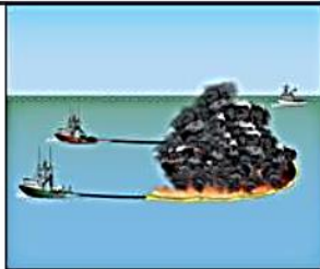
Vessel-based ignition with fire boom for containment
