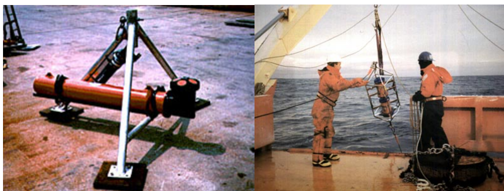
Figure 10. Examples of ADCP's although actual deployment would differ from that pictured above (see description in text).
