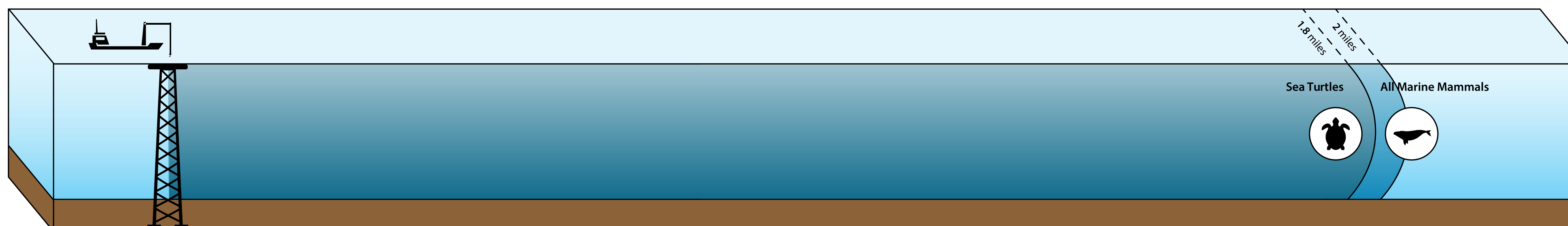
Maximum distances to a 100% adverse behavioral response for marine mammals (160 dB RMS) and sea turtles (166 dB RMS). Distances not adjusted for hearing sensitivity of animal groups shown.
