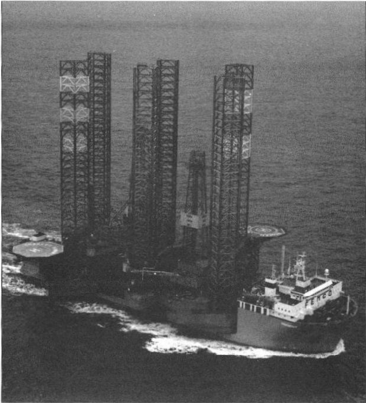
The advent of heavy hauler ships from Western Europe and Russia have enabled mobile offshore drilling rig owners to respond more quickly to changes in world market conditions. Here the Transshelf V carries two large jack-up rigs, the Charles Rowan and the Rowan Juneau , from the North Sea to the Gulf of Mexico.
