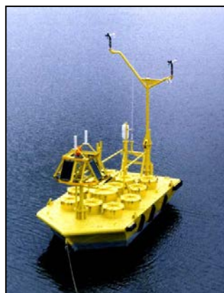
Figure 3-8b 6-meter Boat-shaped Hull Buoy
