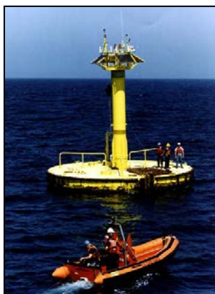
Figure 3-8a 10-meter Discus-shaped Hull Buoy
