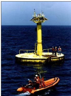
10-Meter Discus-Shaped Hull Buoy , Source: National Data Buoy Center, 2012
