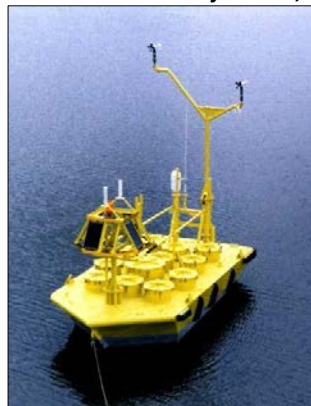
6-Meter Boat-Shaped Hull Buoy Source: National Data Buoy Center, 2012
