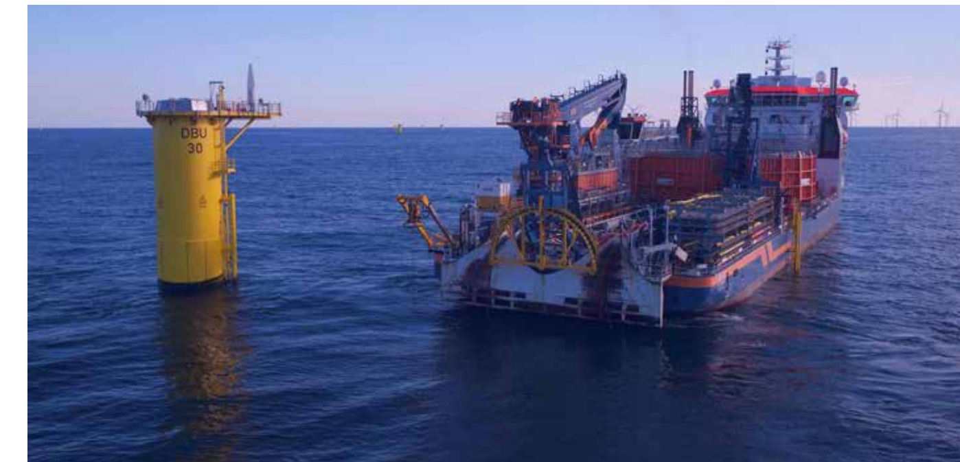
Dynamically Positioned Cable Installation Vessel (Source: Deutsche Bucht and Van Oord)
