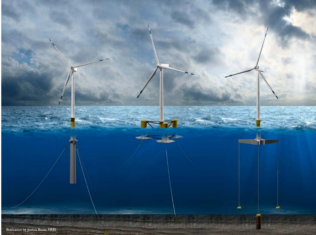
Figure 4. Examples of floating substructure types (left to right): spar, semisubmersible, TLP.
