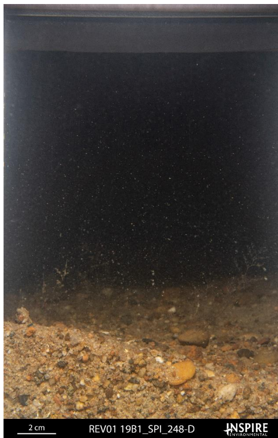
Example SPI and PV Images: Patchy Pebbles on Sand with Mobile Gravel
