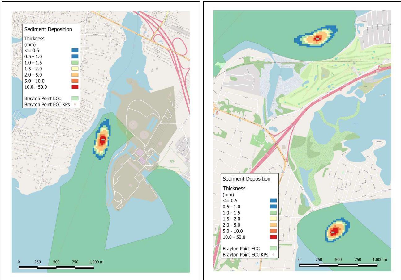
FIGURE 4-19. MAP OF MAXIMUM SEABED SEDIMENT DEPOSITION ASSOCIATED WITH THE EXCAVATION ACTIVITIES AT THE THREE HDD CONNECTION PITS AT BRAYTON POINT (LEFT MAP), AND MOUNT HOPE BRIDGE AND AQUIDNECK ISLAND (RIGHT MAP).
