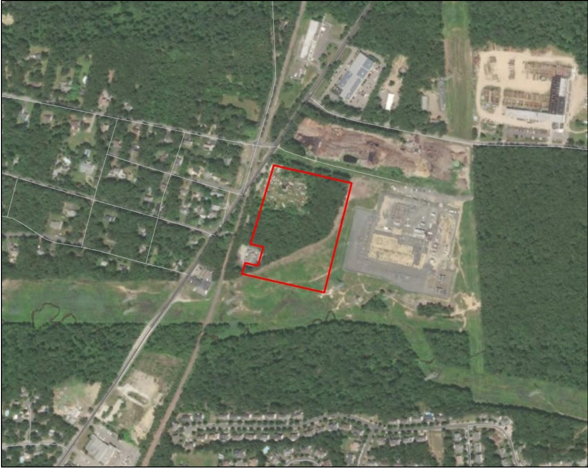
Figure 2.4-1 Aerial view of existing conditions at the proposed substation site (Google Earth, 2020). The substation boundary is shown in red. Note the existing substation immediately to the east.
