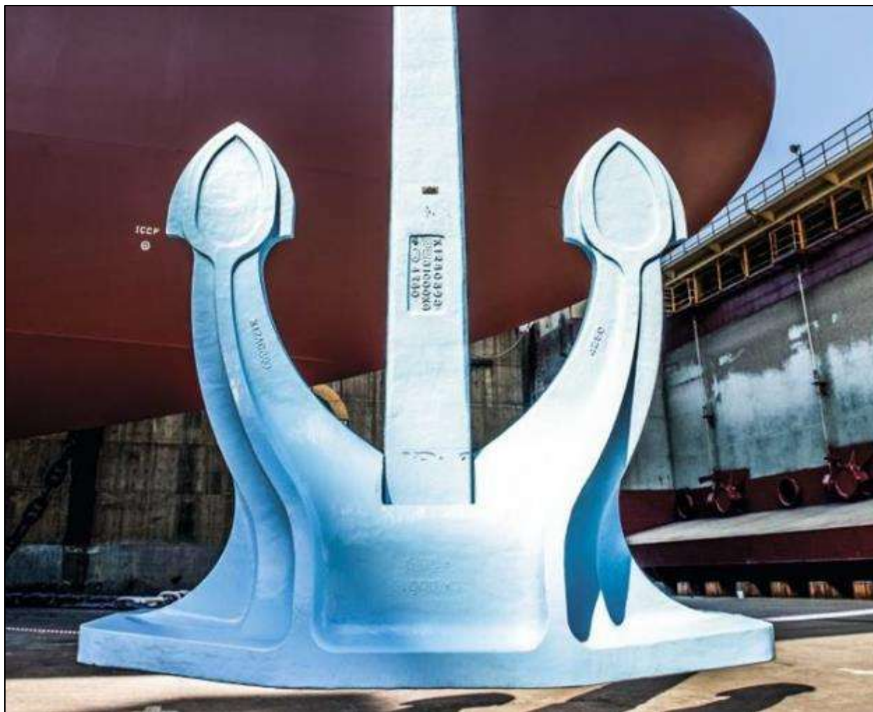
Figure J-19. Maersk Triple E-class Container Ship Anchor (Courtesy of Maersk)
