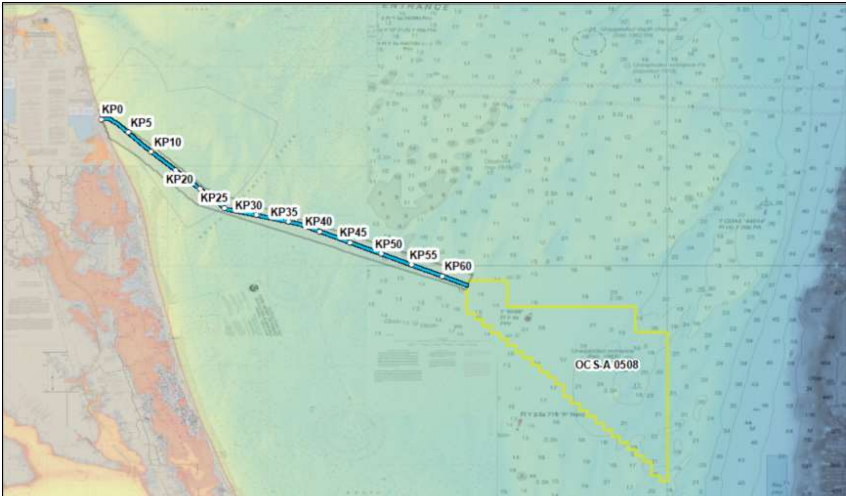
Figure J-5. Overview of the Lease Area and the Offshore Export Cable Survey Area with Kilometer Points (KPs) Marked Along the Offshore Export Cable Corridor Centerline
