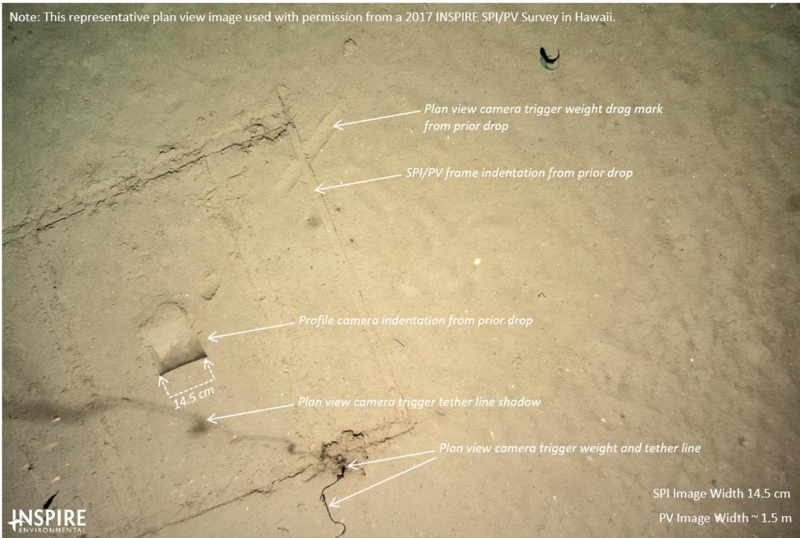
Figure 2.2-2 This representative plan view image shows the sampling relationship between plan view and sediment profile images. Note: plan view images differ between surveys and stations and the area covered by each plan view image may vary slightly between images and stations.
