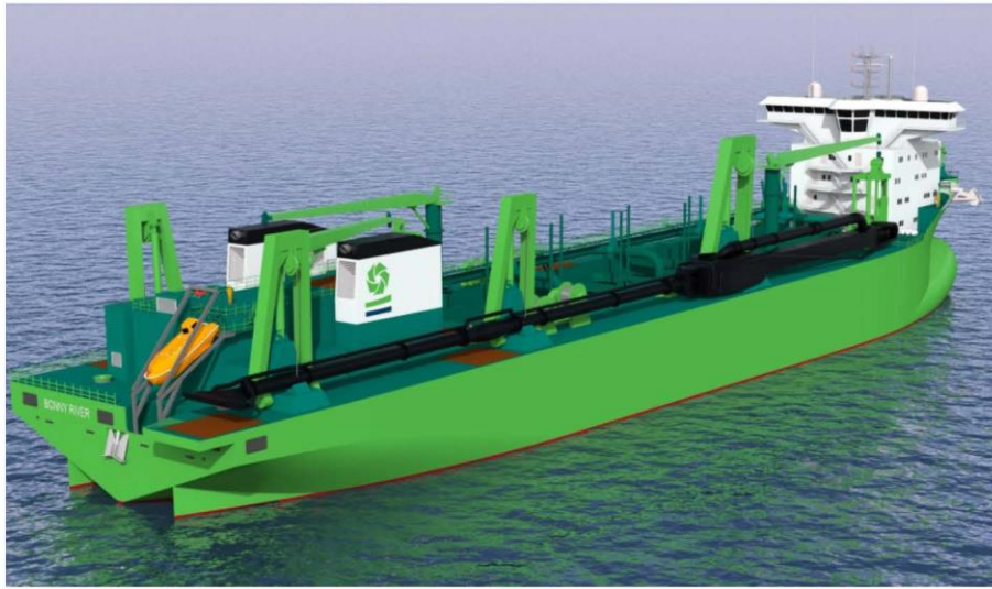
Trailing Suction Hopper Dredge
