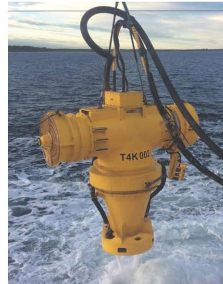
Controlled Flow Excavation
