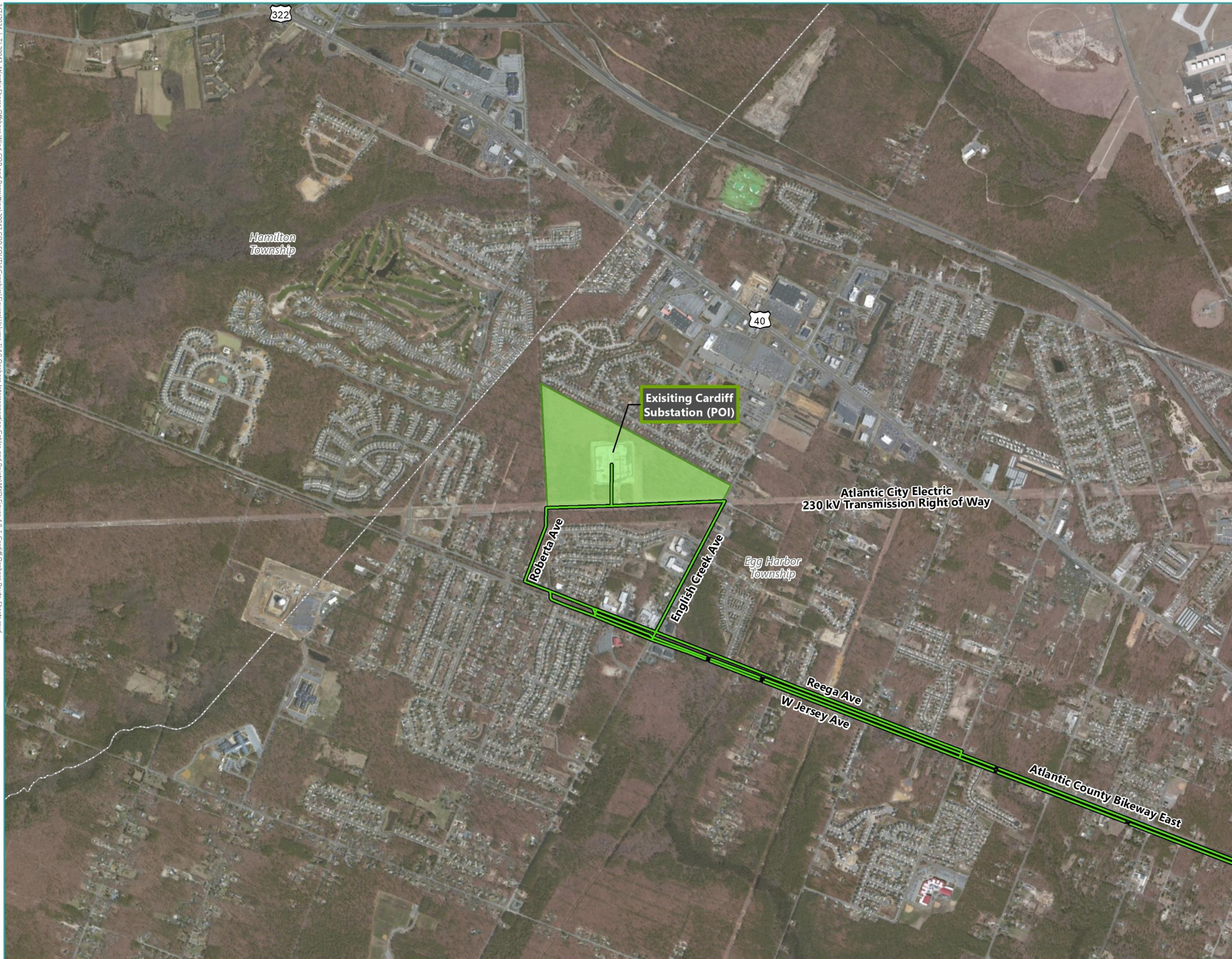
Figure 4.8-1D Atlantic Landfall Site, Cardiff Onshore Interconnection Cable Route, and Onshore Substation Sites Atlantic County, New Jersey
