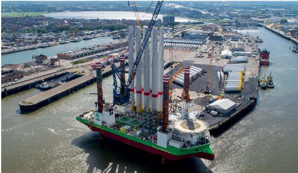
Transport of WTG Components via Jack-Up Vessel
