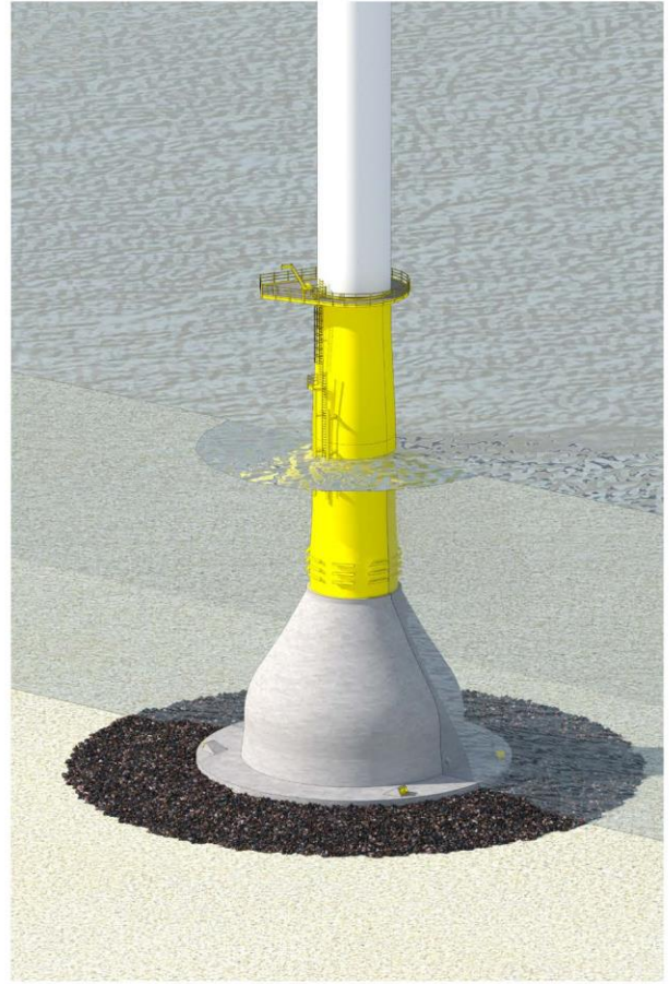
Gravity-Base Structures (GBS)
