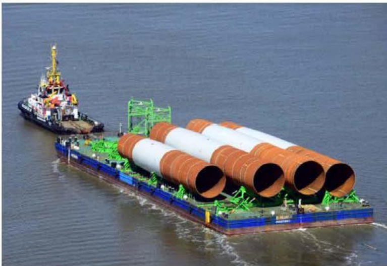
Monopile Transport via Tugboat and Barge
