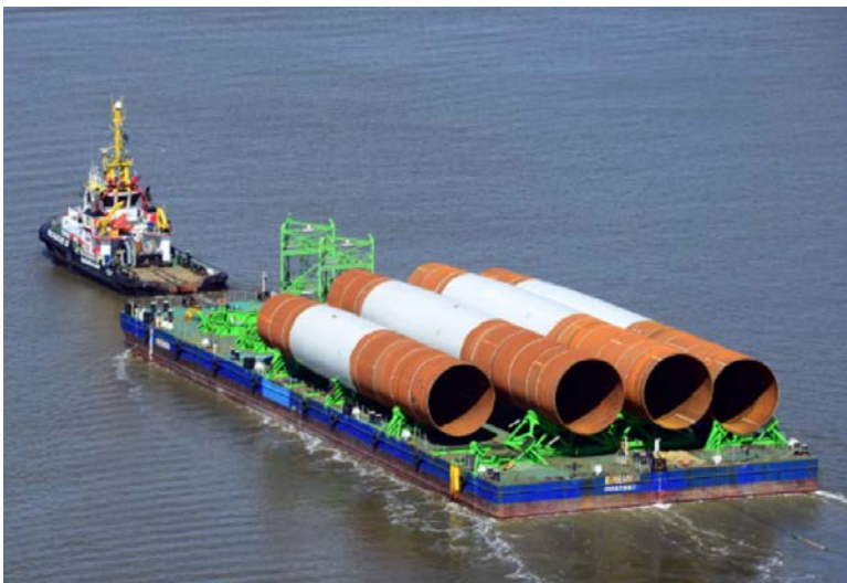
Monopile Transport via Tugboat and Barge
