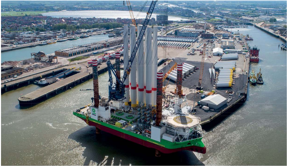
Transport of WTG Components via Jack-Up Vessel
