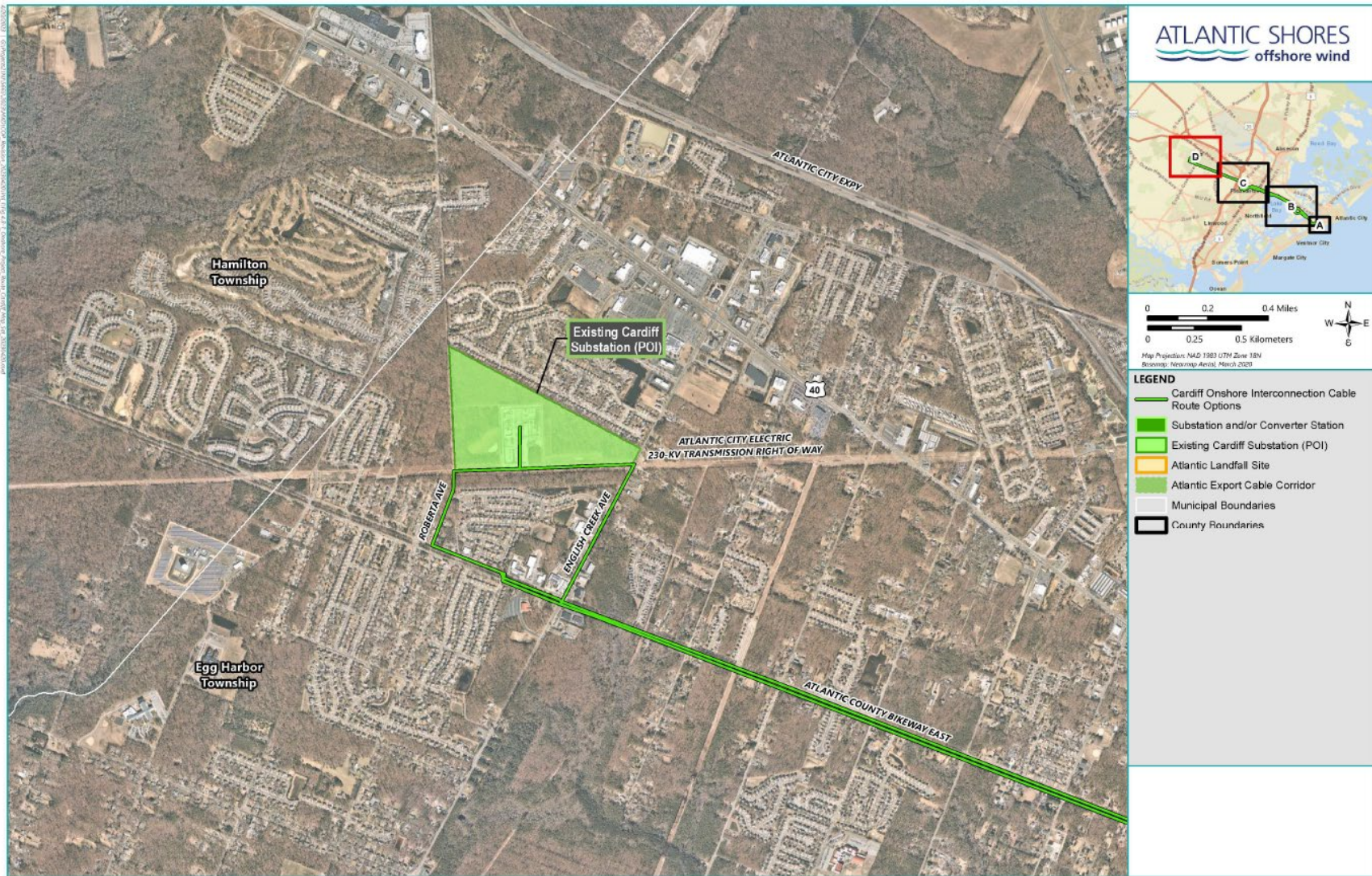
Figure 2-6. Atlantic Landfall Site, onshore interconnection cable routes, and onshore substation and/or converter station sites
