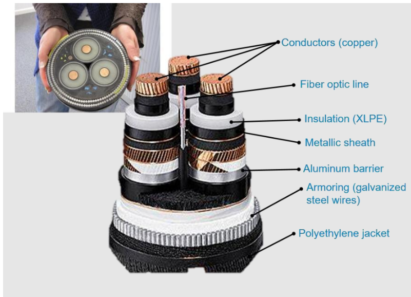
Figure 4. Illustrative Example of an HVAC Submarine Cable.
