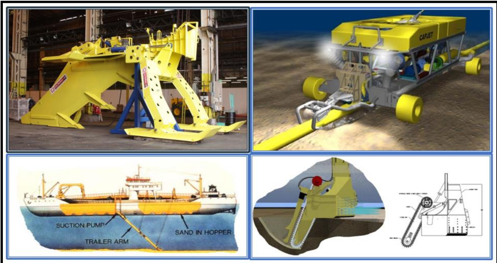
From top left, clockwise: plowing, 32 jetting, 33 trenching (cutting), 34 and suction hopper dredging. 35
