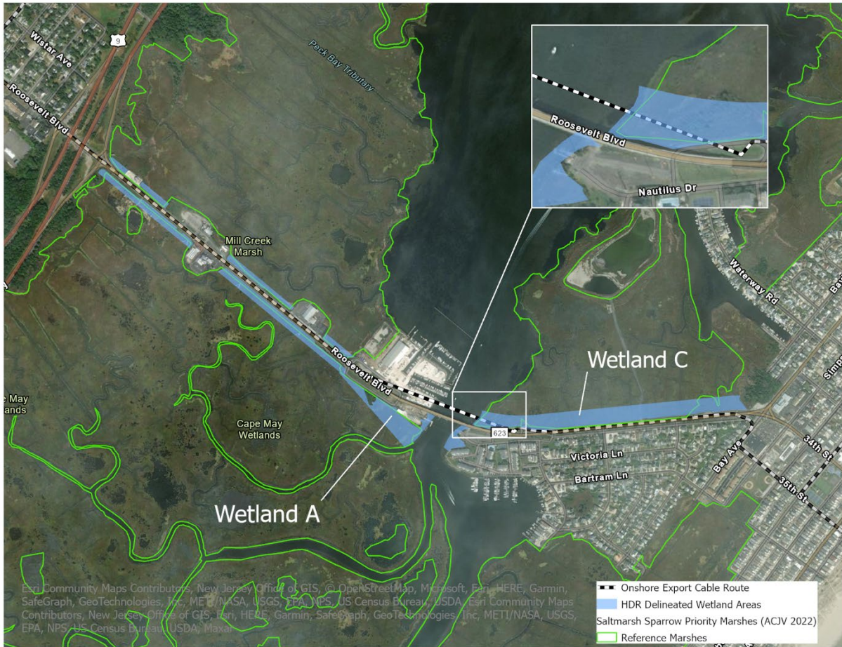
Figure 1: Wetlands A and C delineated up to the edge of the Wetland Review Area. An approximately 94-m segment of the BL England Onshore Export Cable crosses Wetland C. Wetlands A and C delineated by HDR.
