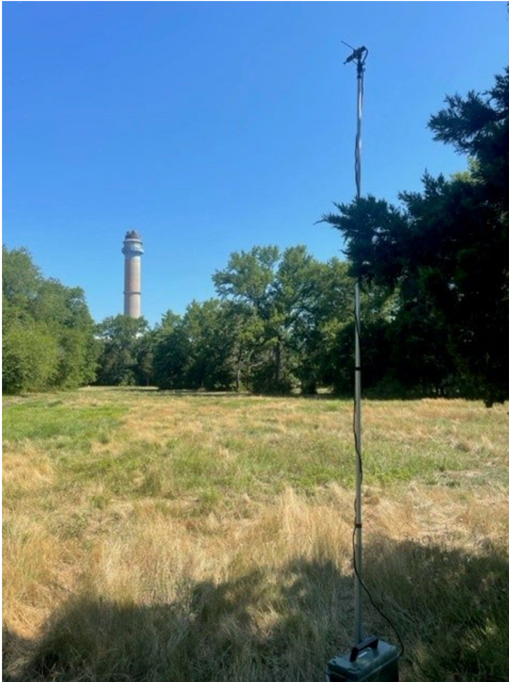
Photo 11. Bat detector and microphone deployment at Site 2 at the B.L. England (BLE) location.
