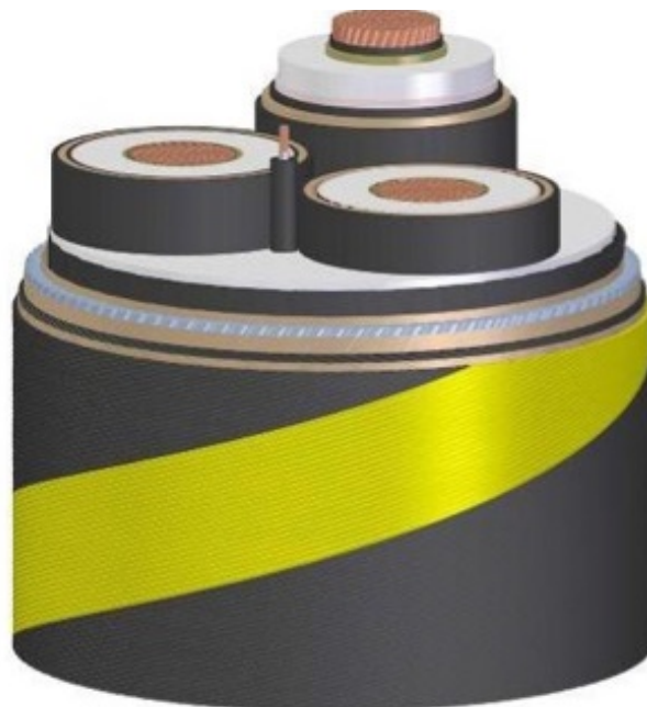
Figure 3.2-1. South Fork Export Cable Cross Section
