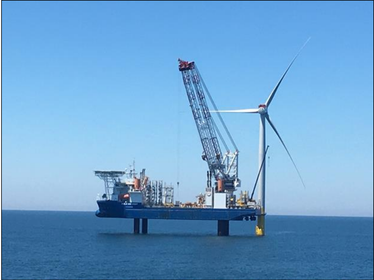
Figure 4.4-67. Example of Wind Turbine Installation Vessel
