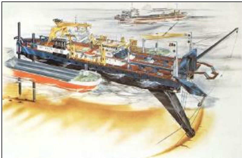
Figure 2.3.2-5. Example of a Cutter Suction Dredge (Frabotta 2012).
