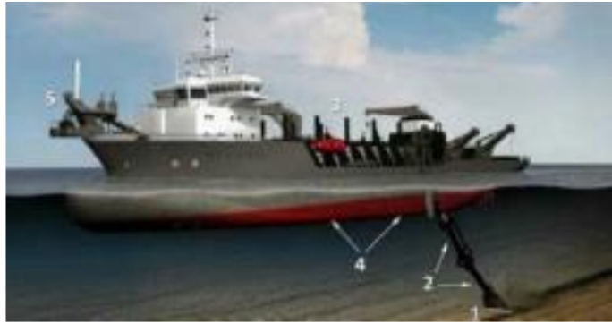
Figure 2.3.2-4. Seafloor Disturbance from a Trailing Suction Hopper Dredge (TSHD). (The TSHD components include a draghead (1), on the end of a large suction pipe (2) through which large centrifugal pumps transport the dredged material as a slurry to the hopper (3) from where it is later discharged either through bottom doors (4) or pumped (5) through a pipeline from the bow) (Michel et al. 2013).
