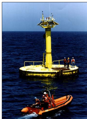
Figure A.3.2-2. 10-Meter Discus-Shaped Hull Buoy (Source: (National Data Buoy Center 2012).
