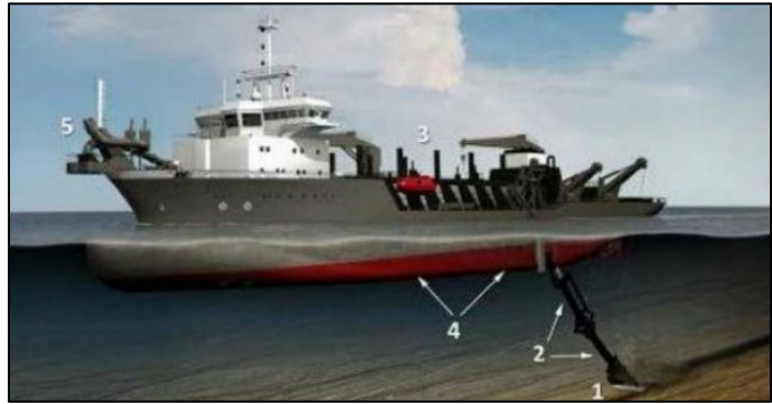
Figure B.3.2-6. Seafloor Disturbance from a Trailing Suction Hopper Dredge (TSHD). (The TSHD components include a draghead (1), on the end of a large suction pipe (2) through which large centrifugal pumps transport the dredged material as a slurry to the hopper (3) from where it is later discharged either through bottom doors (4) or pumped (5) through a pipeline from the bow.) (Michel et al. 2013).
