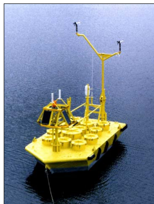
Figure A.3.2-3. 6-Meter Boat-Shaped Hull Buoy (Source: (National Data Buoy Center 2012).
