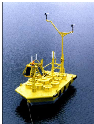
Figure A.4-3. 6-Meter Boat-Shaped Hull Buoy (Source: National Data Buoy Center 2012).
