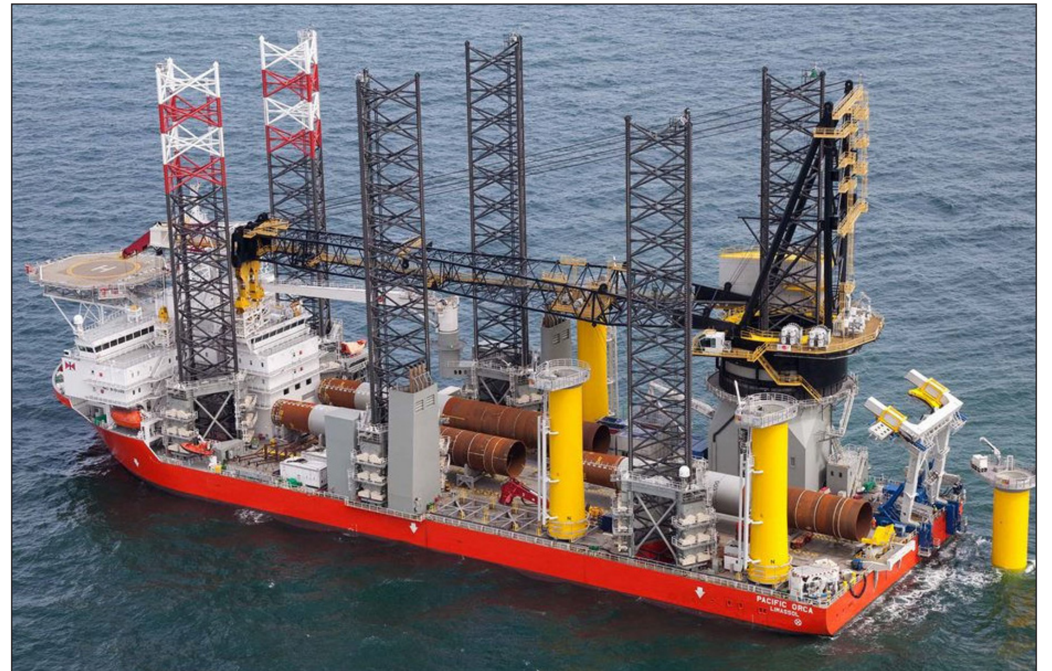
Installation Vessel Pacific Orca loaded with monopiles and transition pieces
