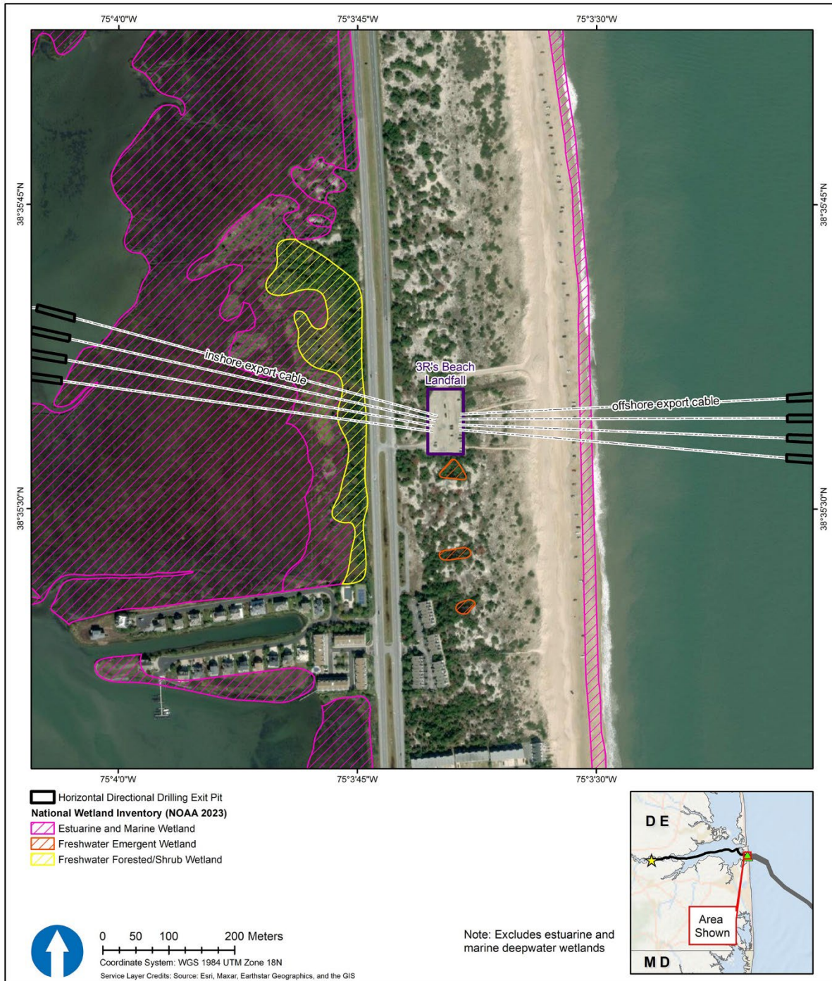
Figure 5-1. 3R's Beach landfall: HDD with offshore/onshore transition vault connection
