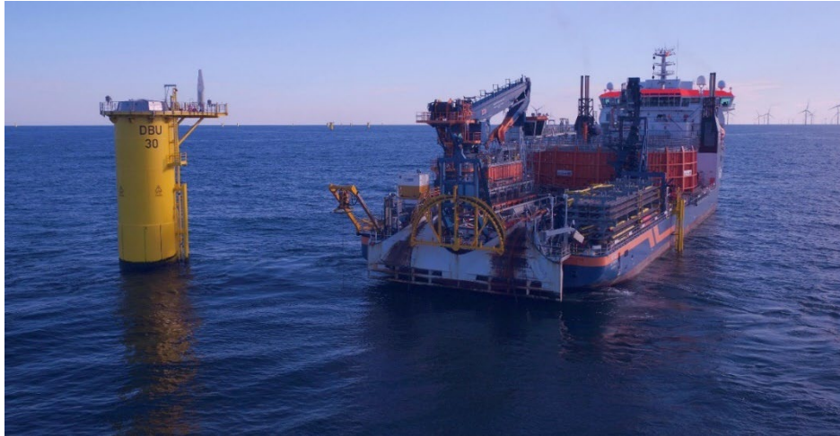
Figure 3-14. Dynamically Positioned Cable Installation Vessel Source: Deutsche Bucht and Van Oord
