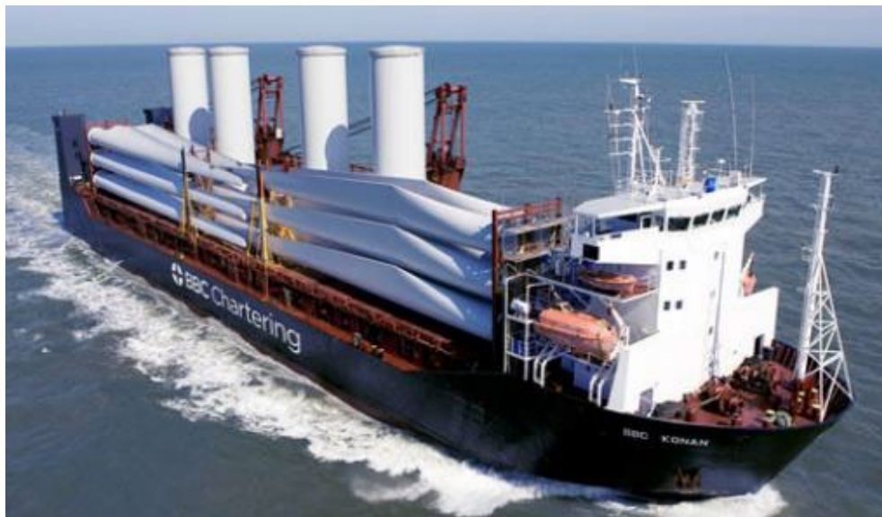
Figure 3-15. Tower Sections Onboard the BBC Chartering and Logistic Ship M/V BBC Konan Source: gcaptain.com
