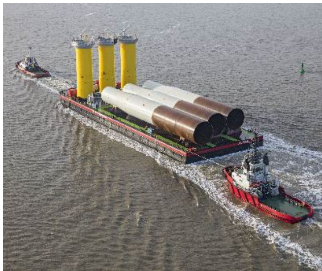
Figure 3-1. Tug and Barge Feeder System for Foundation Transportation
