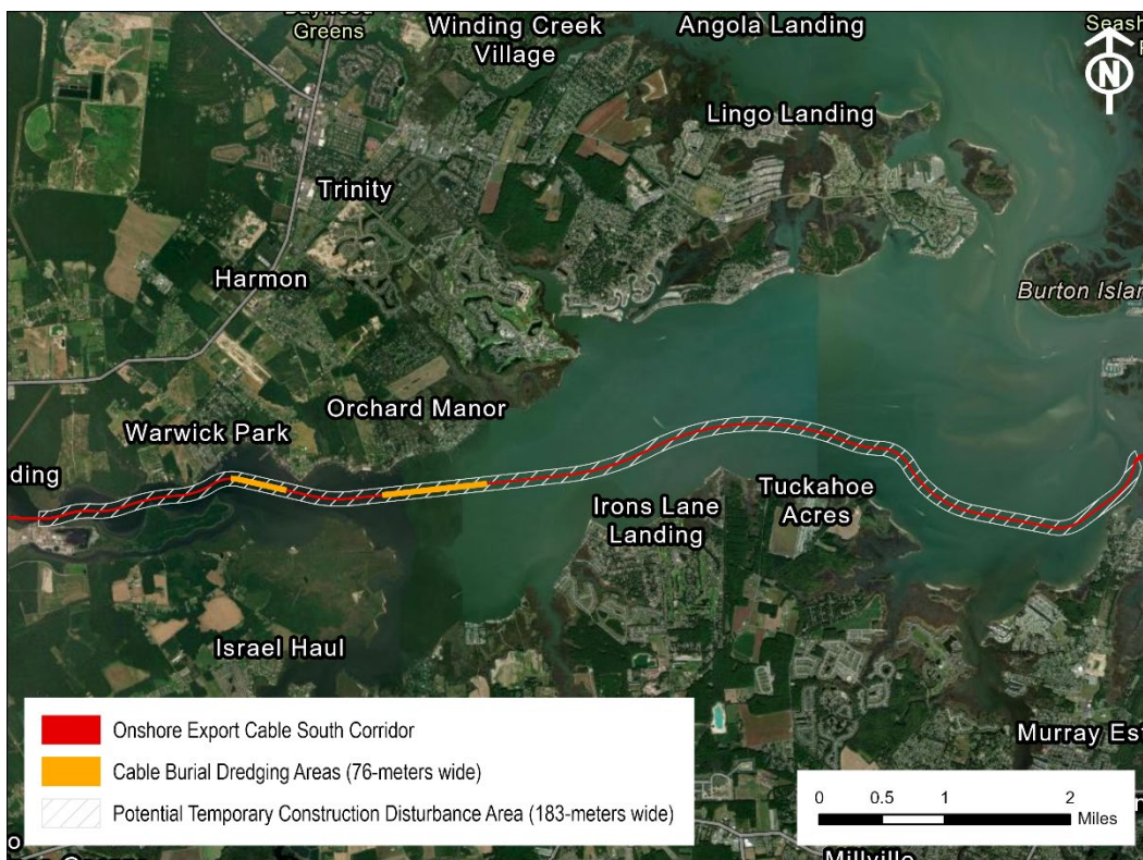
Figure 3-13. Barge Access Dredging Areas within Indian River Bay
