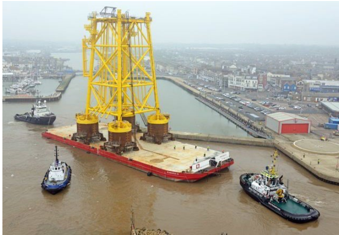
Figure 3-4. Jacket on Suction Bucket Transport
