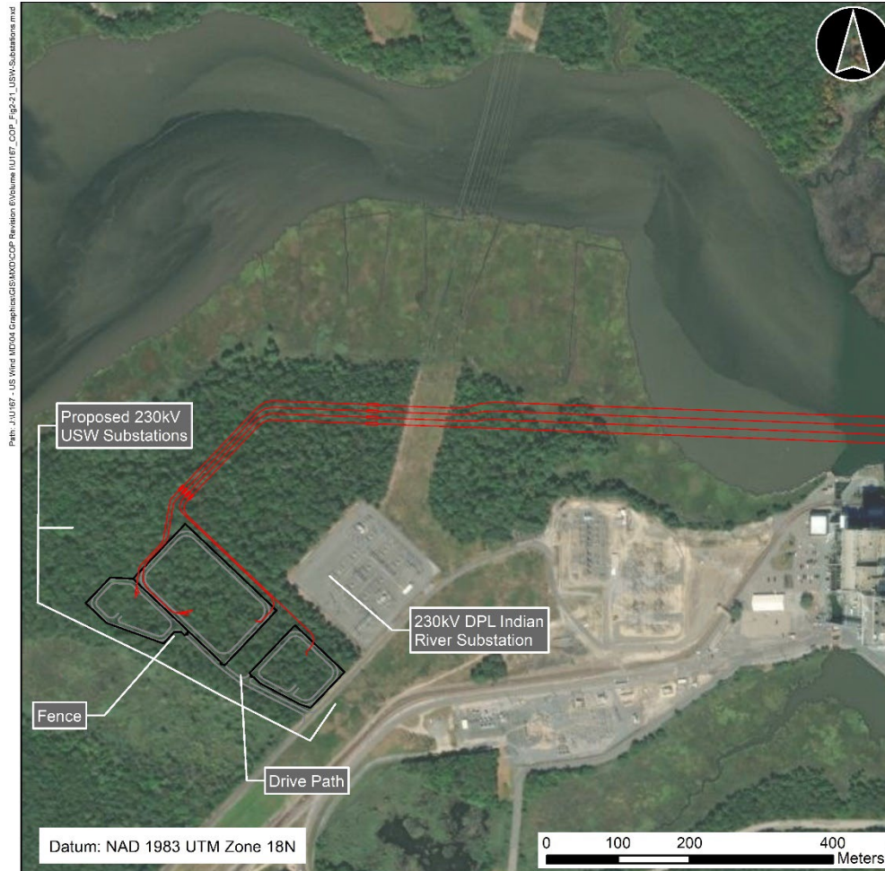
Figure 2-21. DPL Indian River Substation and US Wind Substations (gas insulated)
