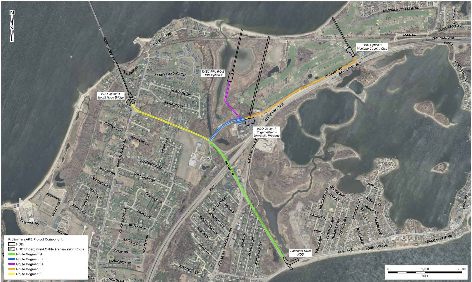
Figure 2.1-2. Proposed onshore cable routes and HDD locations for the Mayflower Wind Aquidneck Island Landfall in Portsmouth, RI.
