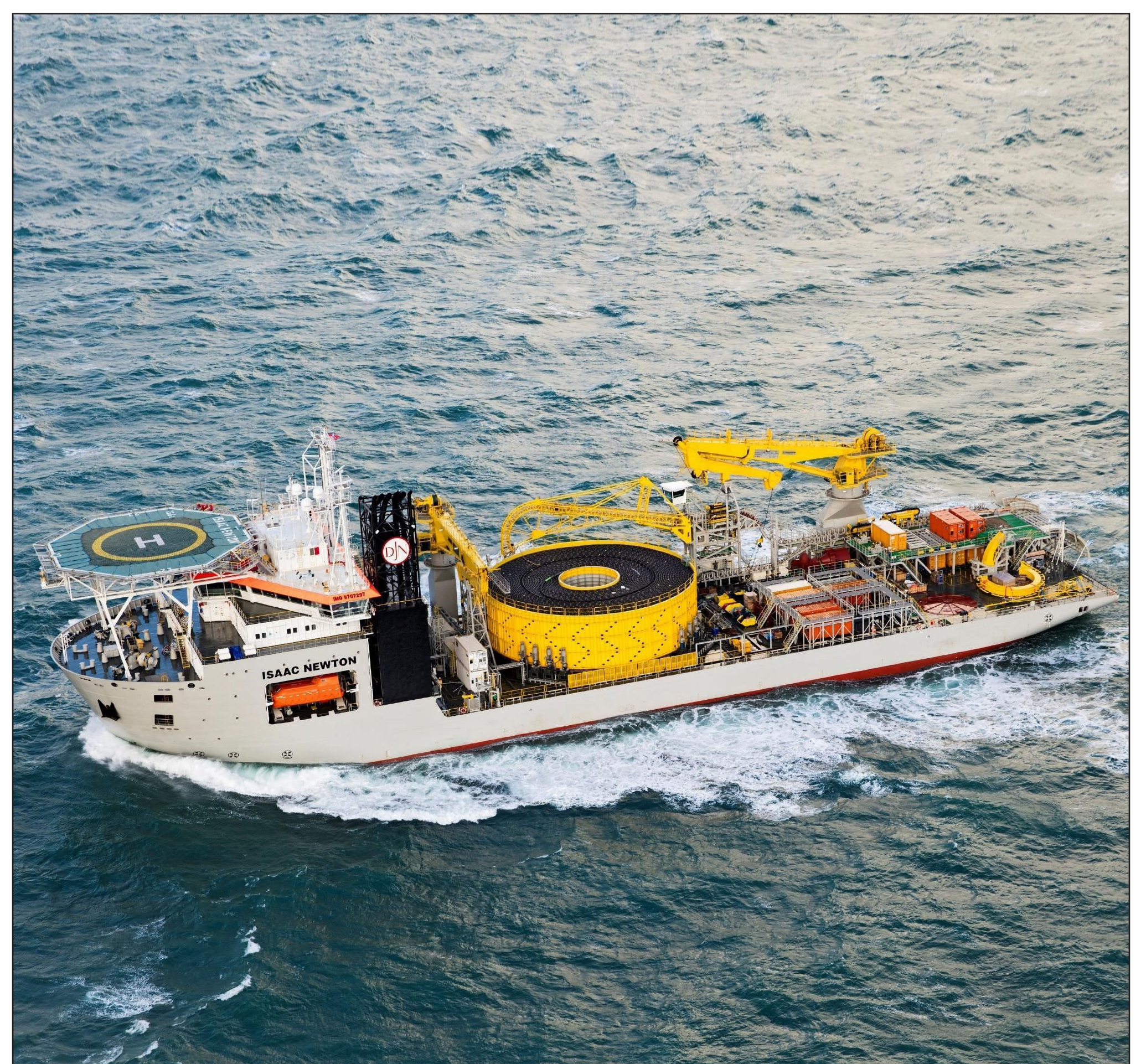
Cable Laying Vessel (Source: Jan De Nul 2020)
