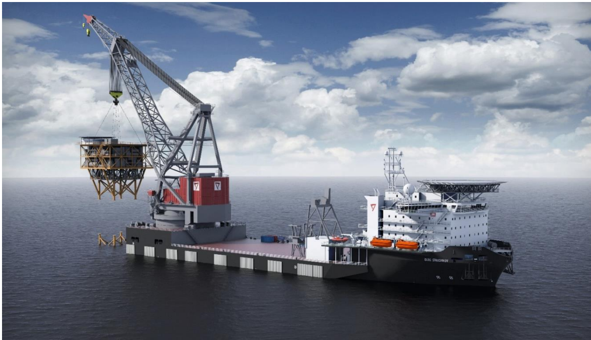
FIGURE 3-18. EXAMPLE OF HEAVY LIFT VESSEL INSTALLING AN OSP
