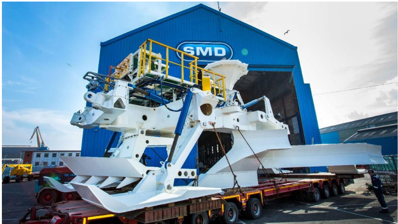
FIGURE 3-22. EXAMPLE OF BOULDER CLEARING PLOW
