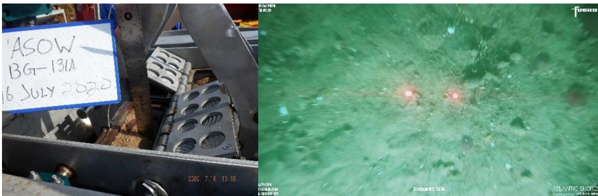
Figure A-63. OCS-20-31: Left image: Grab sample, CMECS: Very Coarse/Coarse Sand. Right image: Seafloor image, complex habitat: no.
