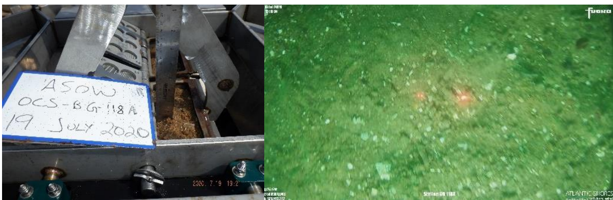
Figure A-55. OCS-20-118: Left image: Grab sample, CMECS: Gravelly Sand. Right image: Seafloor image, complex habitat: yes.
