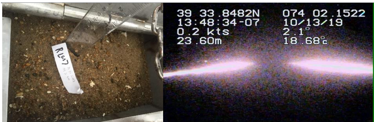
Figure A-6. SOI7: Left image: Grab sample, CMECS Gravelly Sand & Trace Clam Hash. Right image: Seafloor image, taken from 0.46 m above the seafloor; field of view: 0 cm 2 .
