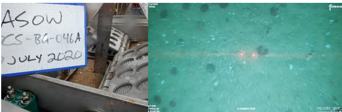
Figure A-33. OCS-20-046 Left image: Grab sample, CMECS: Very Medium Sand. Right image: Seafloor image, complex habitat: no.
