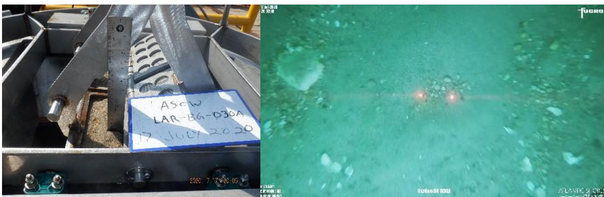
Figure A-25. LAR-20-030 Left image: Grab sample, CMECS: Gravelly Sand. Right image: Seafloor image, complex habitat: yes.
