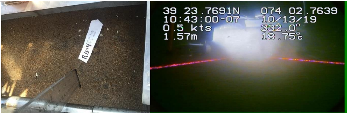
Figure A-3. SOI4: Left image: Grab sample, CMECS Medium Sand & Trace Clam Hash. Right image: Seafloor image, taken from 0.46 m above the seafloor; field of view: 1,393 cm 2 .
