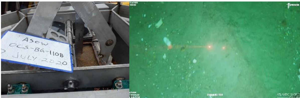
Figure A-49. OCS-20-110: Left image: Grab sample, CMECS: Gravelly Sand. Right image: Seafloor image, complex habitat: yes.
