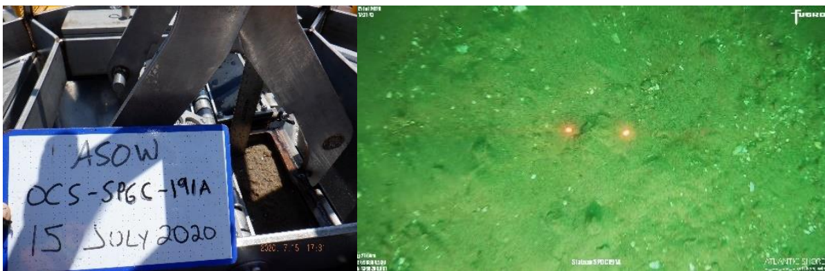
Figure A-72. OCS-20-191: Left image: Grab sample, CMECS: Medium Sand. Right image: Seafloor image, complex habitat: no.
