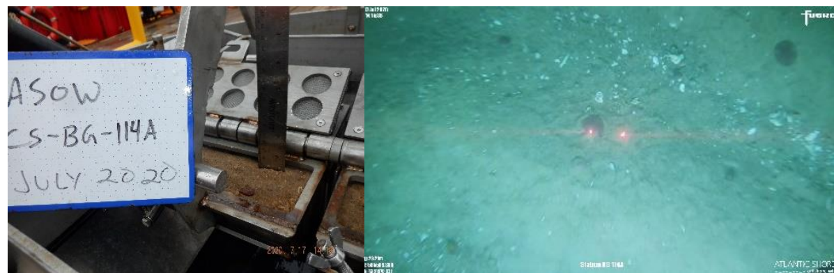
Figure A-52. OCS-20-114: Left image: Grab sample, CMECS: Gravelly Sand. Right image: Seafloor image, complex habitat: yes.
