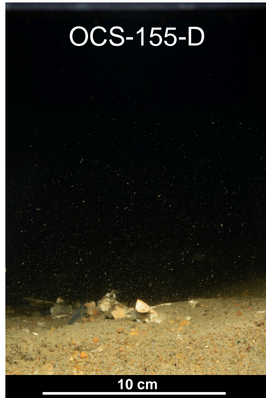
Figure 3-3. Three replicate SPI/PV image pairs from Station 155, showing small-scale heterogeneity grain size at a single station, ranging from very fine to coarse/very coarse sand. Scale: width of SPI images = 14.4 cm; width of PV 155-B = 93 cm, 155-D = 75 cm, 155-F = 78 cm.
