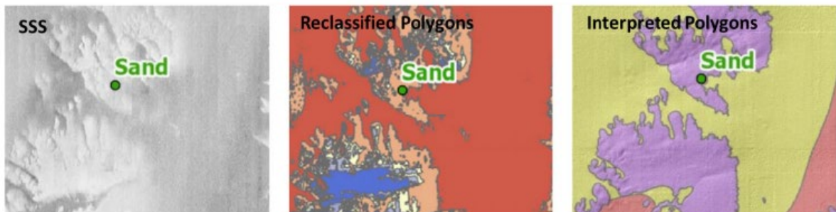
Figure 2.1: Seafloor sediment interpretation, SSS input data (Step 1), reclassification (Step 4), and mapping examples (Step 6) of interpretation workflow
